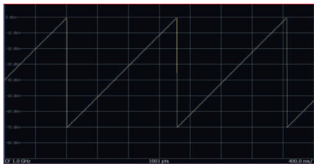
▲ Fig. 3 The continuous power sweep has 70 dB dynamic range.
